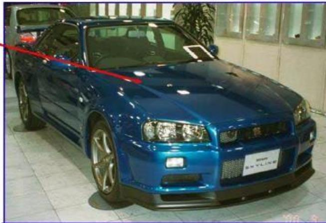
CFRP engine hood (Nissan Skyline GT-R)
